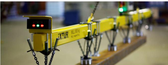
Ixtur lifting beams are fully automatic and cordless. They are battery-powered and do not need an external power supply. The beams' capacities can range from hundreds to thousands of kilograms.
